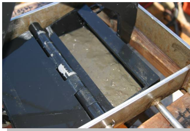
Surficial sediment collected with Van-Veen sampler
