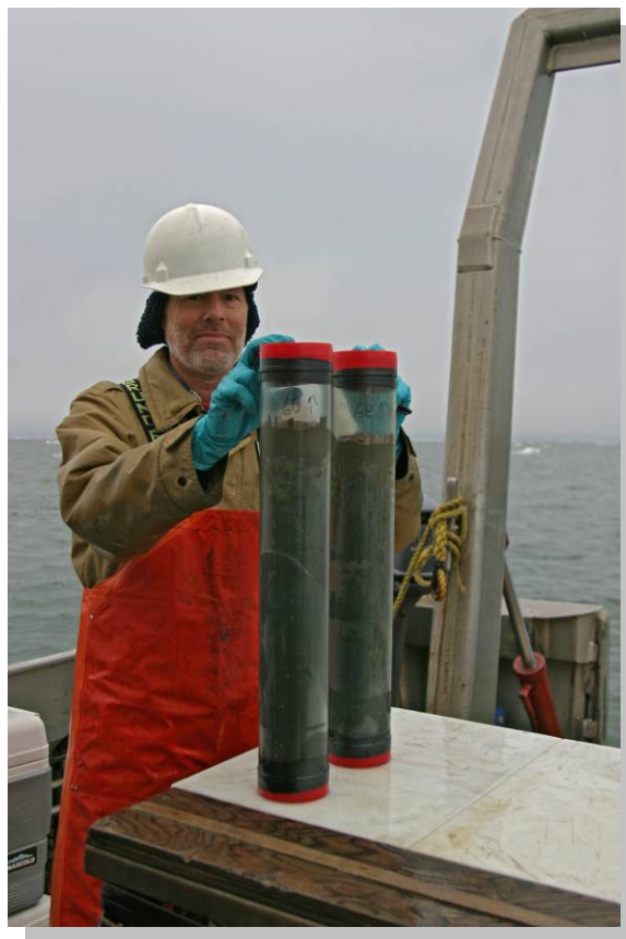
R. Trocine with dual gravity core samples
